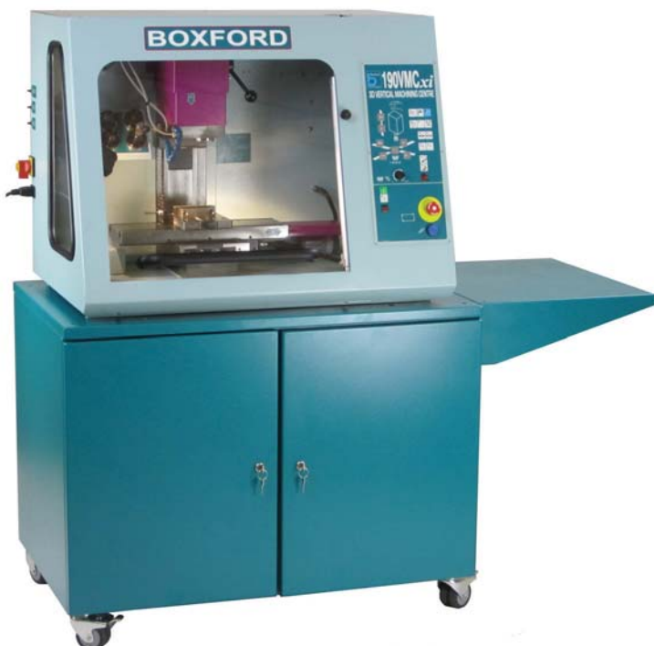
Shown with optional Portable Cabinet Base, Laptop Shelf, Auto Tool Changer, Automatic vice and Air Mist Coolant
